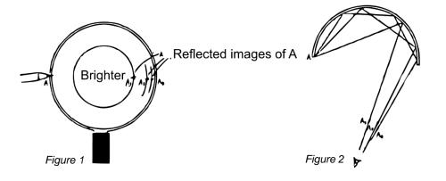
This effect is based on the fact that A1 represents a single reflection of light rays from the surface of the mirror. A2 is a double reflection and A3 is a triple reflection light within the interior of the mirror (see Fig. 2).
