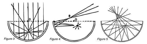
Parallel rays entering the interior of the hemisphere are not completely concentrated at one point, and thus strictly speaking, there is no focal point under this condition, although the rays are concentrated within rather narrow range.
