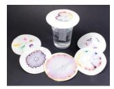
discs allow students to separate most water-soluble inks into their original blended pigments, revealing their hidden identities. Simply make several dots or lines of different colors in the center of the disc using water-soluble markers. Water from a cup is drawn up to the center of a disc using a paper towel. As the water is absorbed into the filter disc the pigments separate into a colorful display.
