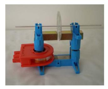
Now spin the disc using the axle so it rotates quickly and whilst spinning briefly connect the coil to a DC power supply delivering 6 volts.
