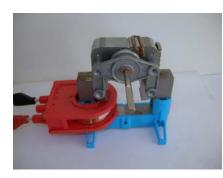
terminals of a 1035411 power supply and apply 12 volts AC you may need to assist the rotor overcome initial inertia by twisting the shaft. Use of the rubber bands supplied to clamp the parts will ensure better operation and quieter running.
