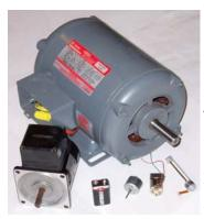
verts electrical power to mechanical power in its rotor (rotating part). In the AC motor this power is induced in the rotating device. An induction motor can be called a *rotating transformer* because the stator (stationary part) is essentially the primary side of the transformer and the rotor (rotating part) is the secondary side. Induction motors are widely used, especially polyphase
