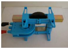
You will need to assist the wheel to spin by turning it fairly hard with the finger to begin rotation under power. This speed should roughly equal the frequency which is 50 Hz. In commercial practice a ca-
