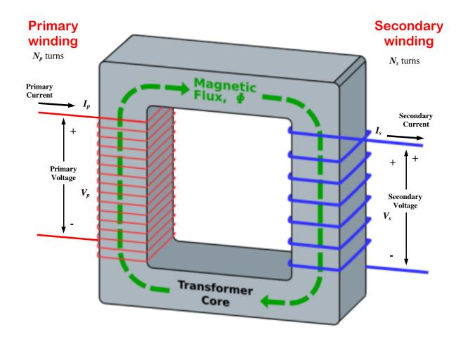
energy to the useful output in the secondary coil.
