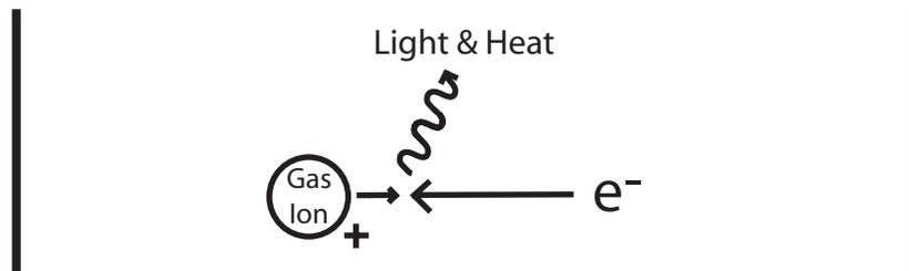
Whenever the charge separation (potential difference) stops or reverses, the electrons recombine with the positive gaseous ions, releasing energy in the form of light and heat. This results in the light that we see from lightning, neon signs, fluorescent lamps, and plasma globes.
