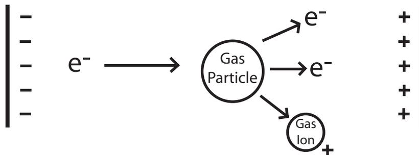
When a charge separation (potential difference) becomes great enough, negatively charged electrons accelerate toward the positive charge. When the electrons travel toward the positive charge, they sometimes collide with neutral gas particles, knocking out negatively charged electrons. This results in positively charged gas particles called ions, as well as extra free electrons.
